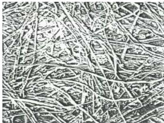
Figure 12. Eraser residue from a MAGIC-RUB block eraser magnified 100 times. Residue and fiber damage are relatively low.
